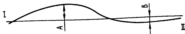
Fig. 4-19. Shock Absorber Performance Curve: I - rebound stroke force; II - compression stroke force
